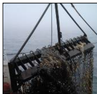
Figure 14. Photograph of twine top hung on turtle guards
