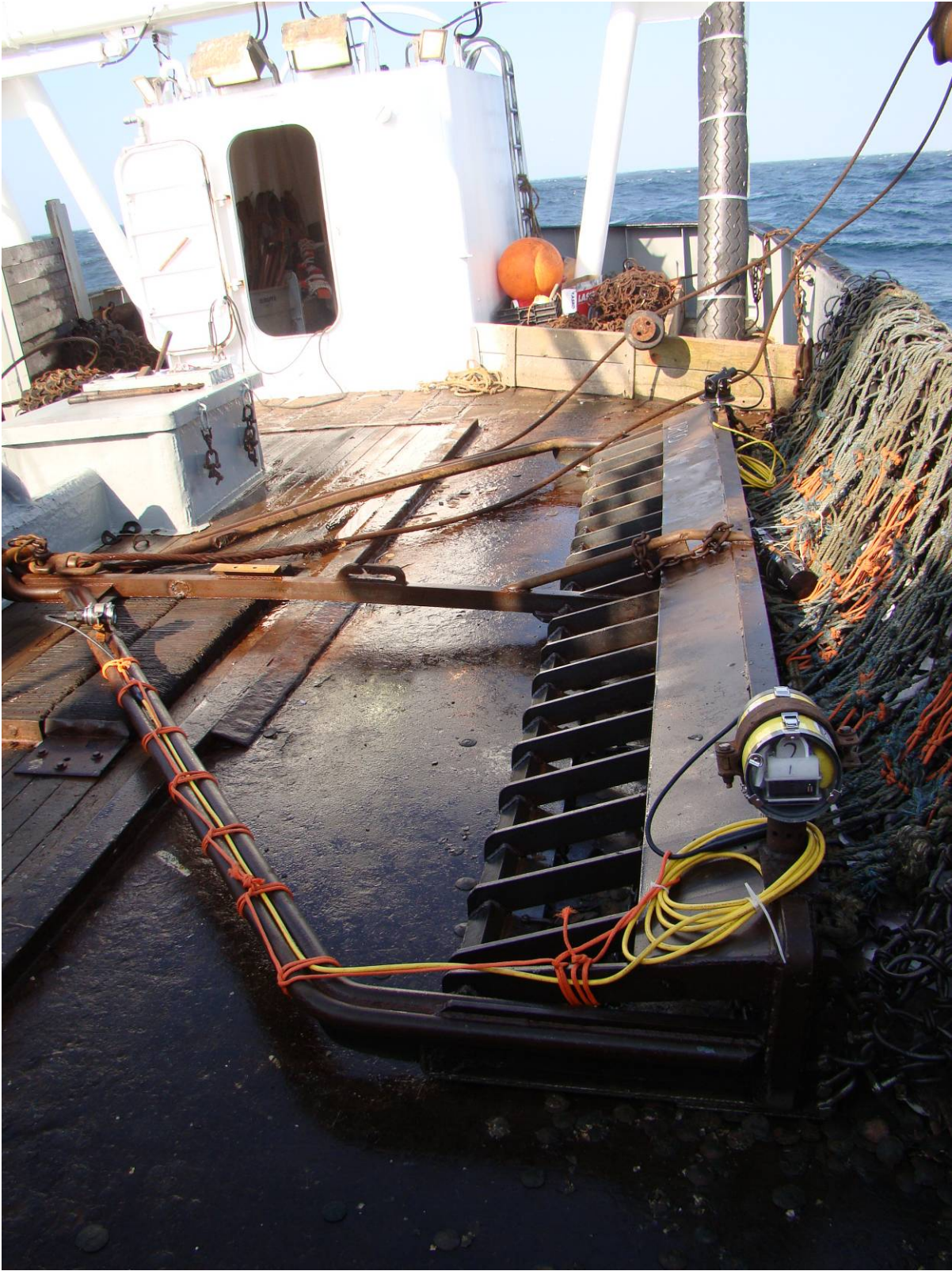
Figure 1: Low-profile dredge showing the placement of cameras during video trials.
